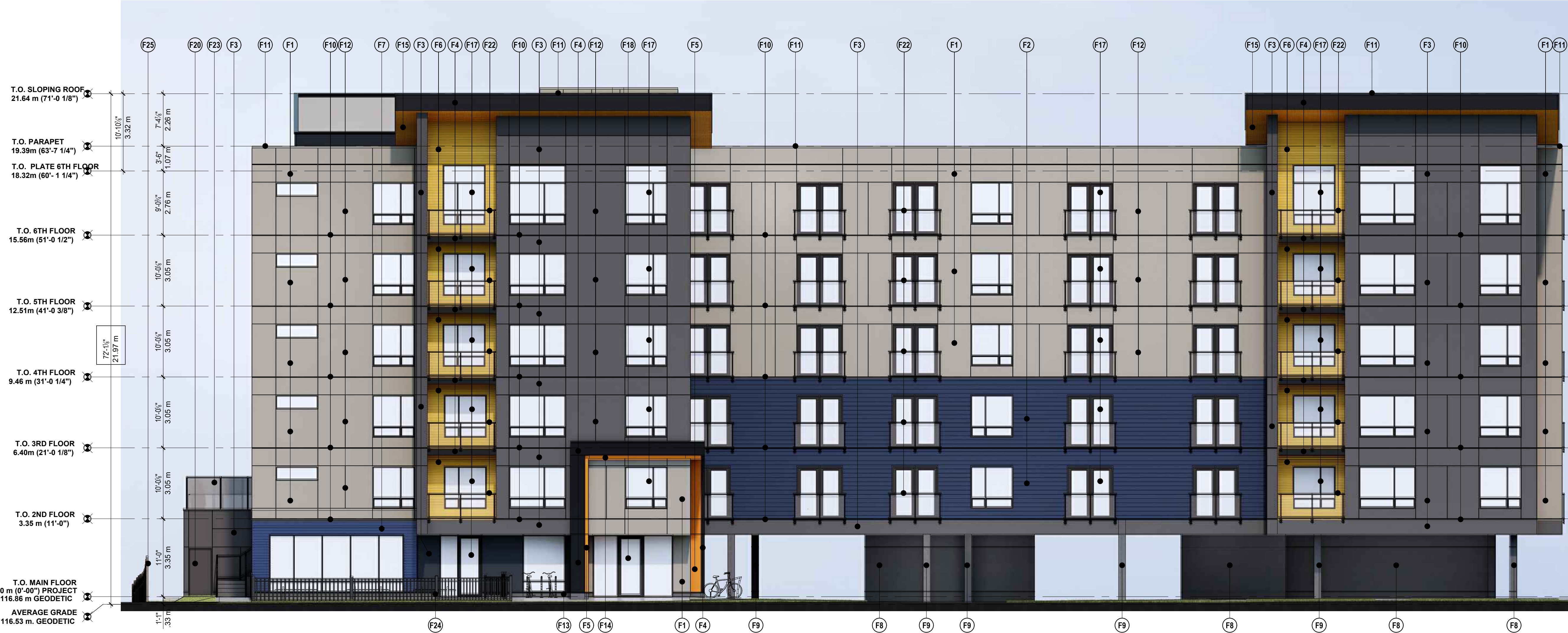
1 NORTH ELEVATION (AT VICTORIA AVENUE) SCALE: 1/8" = 1'-0"
